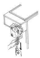
Figure L Remove Plunger and Spring
